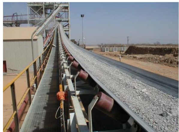
Ore being conveyed from stockpile to grinding mill and processing plant
