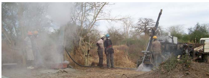
Fig. 17 Rotary Air Blast Drilling Diba Project, Mali Source: Analyst
